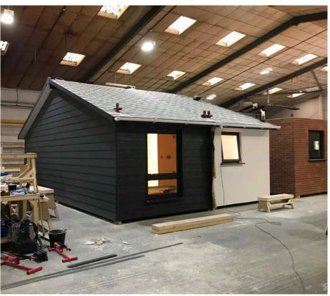
Once the foundations for the building are complete the individual units assembled together in the factory can be separated and delivered to site. Each section of building weighs in at an average of 5.2 ton, so basic crane lifting is all that is required to lift into place.
